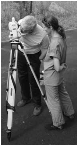
BG Map training instructor Mark Glicksman demonstrates Total Station surveying equipment for assistant gardener Evonne O'Dwyer.
